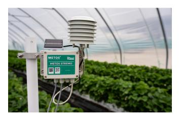
Thank you for choosing a METOS Stremo station for monitoring your agrometeorological conditions. METOS Stremo has been designed for real-time monitoring of plant stress and environmental conditions using a set of advanced sensors that measure leaf transpiration, incident sun light, air temperature, relative humidity and vapour pressure deficit (VPD).
