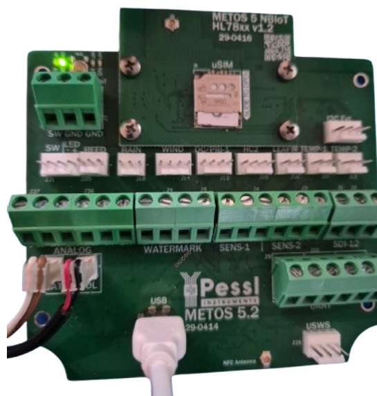
Connected power, inserted SIM card, and connected USB cable.
