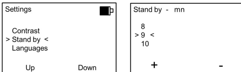
When the Dualex enters the standby mode, all measurements and settings are saved. When you restart the device by a long press on the button
