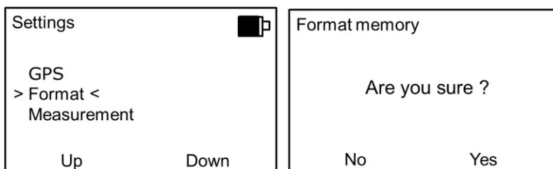
If the buttons (No) or are selected, the data are left intact and the software returns to the main menu.
