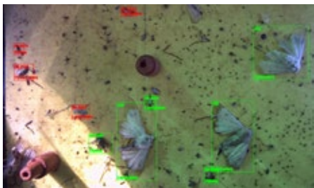
iSCOUT uses automatic recognition algorithm for recognizing pests.
