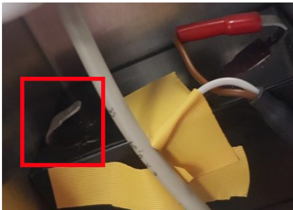
Picture: Connect the battery cable to the free connector (minus, white cable with connector). Battery must always be unplugged transportation purposes.
