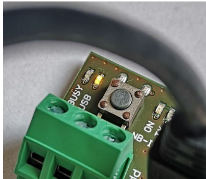
Picture 14 – USB LED status: orange when the USB is connected
