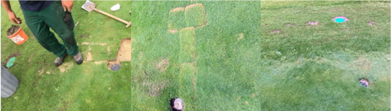
Insert the lawn tile - re-install the lawn tiles to cover sensors 14 days later - "invisible"
