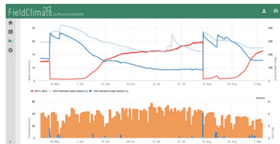
Combination of volumetric water content with two different depths (blue and light blue) and tensiometric data (red) measurements in one Pinot Noir adult vineyard. You can see the succession of drying and potential deficit phases, mitigated by irrigations and rains.
